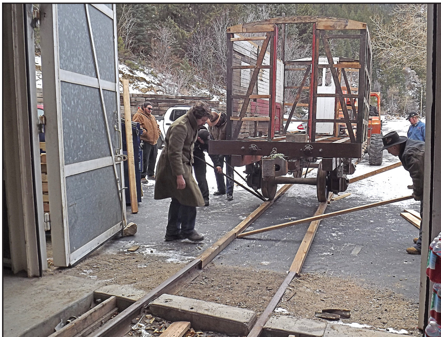
The caboose was very slowly pushed on the wooden rails up to the rails of the Georgetown Loop RR Museum Building. – Photo © 2021 Shane Schabow.
